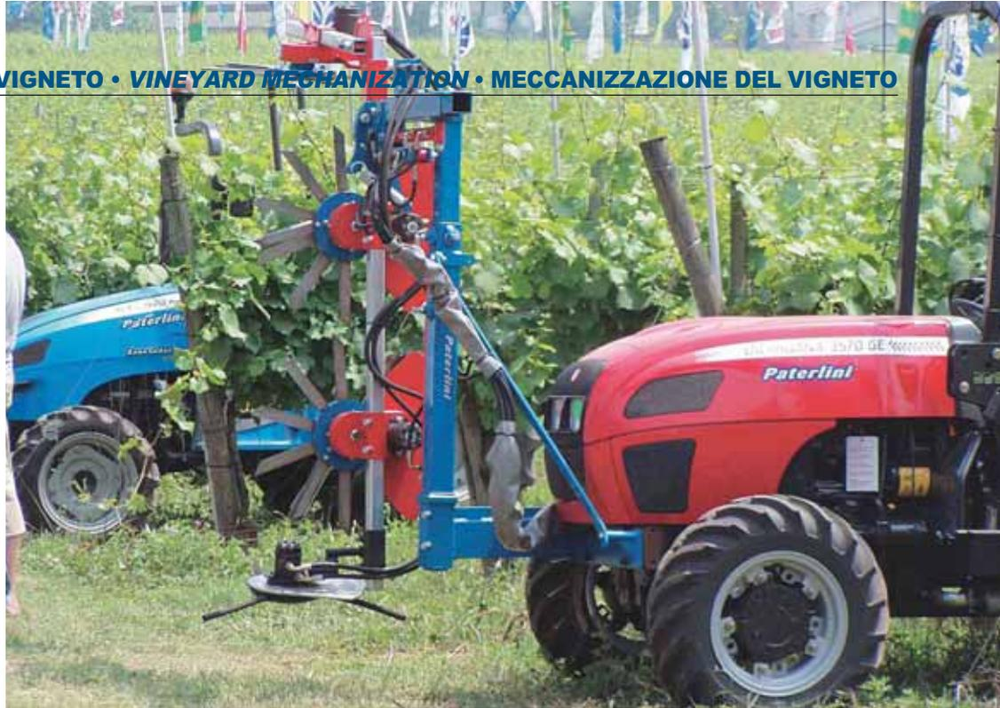
the tractor, whose wheels otherwise risk ripping off the foliage still to be trimmed, although some models offer 'conveyors' to lift and guide the shoots into the cutting blades. Row straddling trimmers work on the two sides of a row at once, but they create problems because the operator cannot see both sides.
